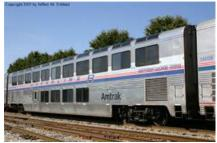
First Amtrak cars to have onboard waste treatment and disposal that linked to all toilets aboard. The trains have both lower and upper level- seating. They use overhead luggage compartments.
