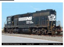
Full name is General Purpose 40. It was manufactured by General Motors' Electro-Motive Division (EMD) between November 1965 and December 1971. The EMD produced 1,221 units. Its engine is an EMD 64E3 and generates 3,000 horsepower. It is distinguishable by the three 48-inch radiator fans that are located in the back of the long hood.
