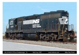
Full name is General Purpose 40. It was manufactured by General Motors' Electro-Motive Division (EMD) between November 1965 and December 1971. The EMD produced 1,221 units. Its engine is an EMD 64E3 and generates 3,000 horsepower. It is distinguishable by the three 48-inch radiator fans that are located in the back of the long hood.
