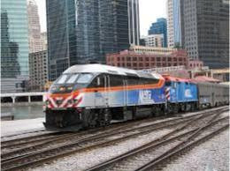
MP36PH-3S: This was the first version built and was only built for the Chicago Metro it is turbocharged, 3600 horsepower, 16 cylinder, is 70 Ft long, and has a top speed of 88 mph. This version uses a series of static (hence the S in the name) invertors which reduce the power needed to move the train. This series was built from 2003-2004
