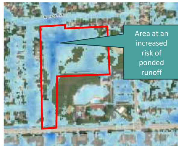
Figure 22: Gouin Park with Modeled Flood Depth and Inundation for the 10-Year Event
